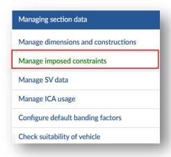
Use **Manage imposed constraints** to add, edit or view imposed constraints associated with a structure as shown below.
